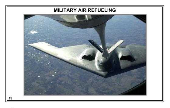
Aerial refueling is a procedure used by the military to transfer fuel from one aircraft to another during flight.
